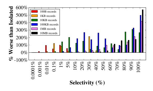
(a) The effect of simultaneity on sequential scans.
