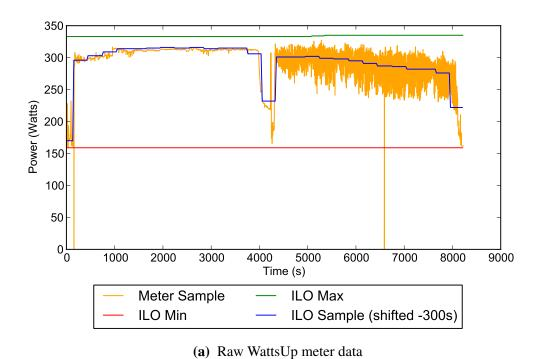
Power (Watts) 0 Time (s) Meter Sample (30s medians) **ILO Max ILO Min** ILO Sample (shifted -300s)
