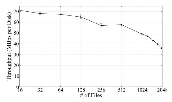
**Figure 4.1.** Performance of the Heaper-Merger sort implementation in microbenchmark on a 200GB per disk parallel external merge-sort as a function of the number of files merged per disk.
