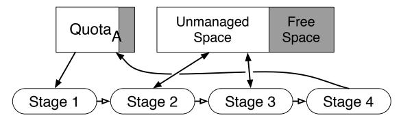
**Figure 5.4.** A diagrammatic overview of quota-based memory management. In this figure,  $Quota_A$  provides a memory quota between Stage 1 and Stage 4. Stages 2 and 3 use unmanaged memory created with standard malloc and free syscalls.
