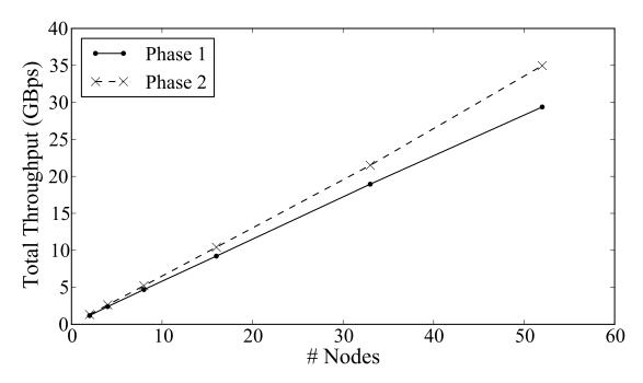
**Figure 4.11.** Throughput when sorting 1 TB per node as the number of nodes increases.
