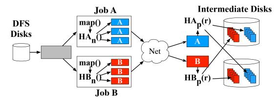
**Figure 6.5.** An overview of multi-tenancy in Themis. Input records are mapped by both job A and job B's map functions, and intermediate records are routed based on each job's partition function independently.
