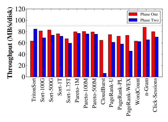
**Figure 5.6.** Performance of evaluated MapReduce jobs. Maximum sequential disk throughput of approximately 90 MB/s is shown as a dotted line. Our TritonSort record from 2011 is shown on the left for comparison.
