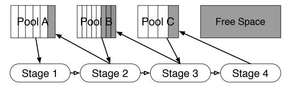
**Figure 5.3.** A diagrammatic overview of pool-based memory management. Note that memory in each pool is divided into fixed-size regions, and that any memory not allocated to pools cannot be utilized by stages.
