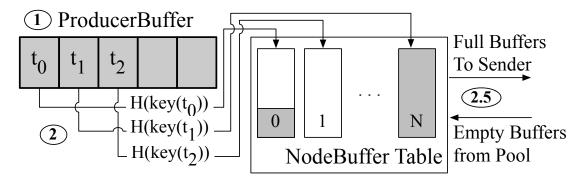
**Figure 4.3.** The NodeDistributor stage, responsible for partitioning records by destination node.
