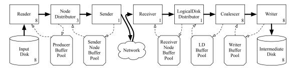
**Figure 4.2.** Block diagram of TritonSort's phase one architecture. The number of workers for a stage is indicated in the lower-right corner of that stage's block, and the number of disks of each type is indicated in the lower-right corner of that disk's block.
