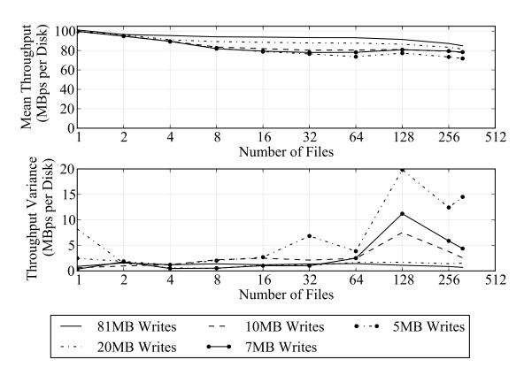
**Figure 4.9.** Microbenchmark indicating the ideal disk throughput as a function of write size.
