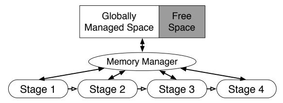
**Figure 5.5.** A diagrammatic overview of constraint-based memory management. All stages' memory requests are satisfied by a central memory manager that schedules these requests according to the stage graph's structure.
