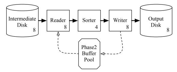
**Figure 4.7.** Block diagram of TritonSort's phase two architecture. The number of workers for a stage is indicated in the lower-right corner of that stage's block, and the number of disks of each type is indicated in the lower-right corner of that disk's block.
